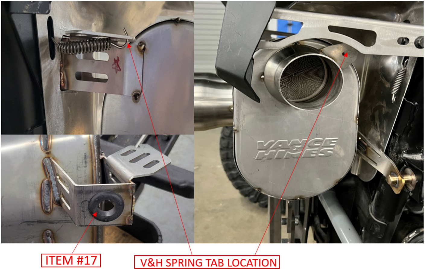
FIG 6: V&H MIDPIPE AND CLAMP
