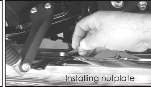
1. Attach mounting bracket 390-P to transmission and tighten to 12-15 Ft/Lb torque. (Figure 1). NOTE: 2006 to 2007 models use three 5/16" x 1-1/2" hex head bolts and washers. 2008 to 2011 models use three 5/16" x 1-1/2" hex head bolt, washers, 11/16" spacer between the bracket and transmission in top hole. 2012 and later models use one 5/16" x 2" hex head bolt, washers 11/16" spacer in top hole and two 5/16" x 1-1/2" hex head bolts and washers in remaining holes.
